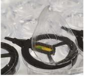
Take the sample holder off the cavity and screw it into an XtalTool Base (Cat. No. X-XT-105) until the indication marker is reached.
