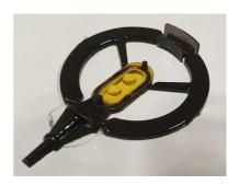
2. Flip over the sample holder and place it onto a greased cavity of a 24 well plate. The design is such that 24 sample holders will fit onto the plate.
