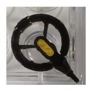
3. Seal the cavity with the sample holder. Ensure that XtalTool HT is placed correctly indicated by the two outer positioning guides on either side.
