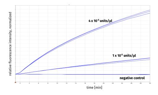
Kinetic evaluation of DNase I activity monitored on the real-time PCR system QuantStudio 5 (ThermoFisher). Concentration of DNase I standards are 1 x  $10^{-5}$  units/ $\mu$ l and 4 x  $10^{-5}$  units/ $\mu$ l. PCR-grade water is used for negative control.
