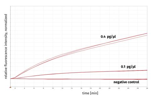
Kinetic evaluation of RNase A activity monitored on the real-time PCR system QuantStudio 5 (ThermoFisher). Concentration of RNase A standards are 0.1 pg/ $\mu$ l and 0.4 pg/ $\mu$ l. PCR-grade water is used for negative control.
