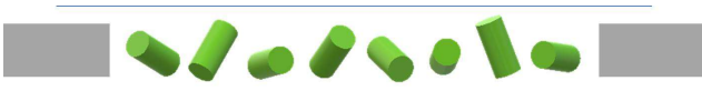
Fig. 1 Schematic cross section of a grid hole with ideally distributed single particles in random orientation
