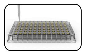
Step 3. Position the 200 Micron UV Cover Film onto the 96 wells and check integrity. N.B. Please ensure the protective film is facing up.
