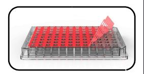
Step 2. Load up to a maximum of 3200 nanolitres (up to 3.2µl) protein into each well.
