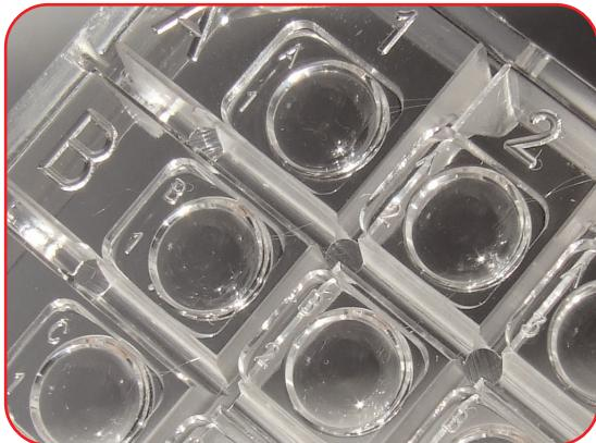
The new MRC Under Oil 96 well Crystallisation plate uses proprietary oil specially selected for the purpose of running macromolecular crystallisation under oil. Following the initial experiment, the solution under the oil is sequentially allowed to evaporate as a second stage enabling further crystal growth as a consequence of concentration.
